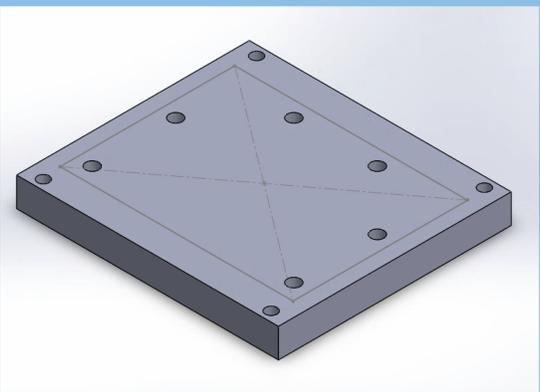
Figure 4 – Conversion Plate Between C and Nozzle Fixture
